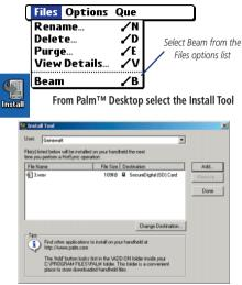
Files added to the Install Tool are sent to the SD Card when you perform a HotSync® operation.
